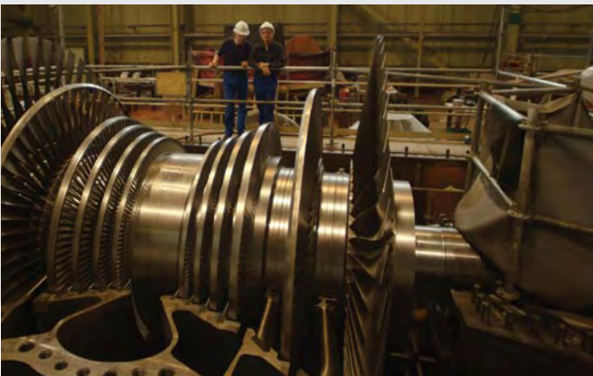
Turbine replacements improve plant efficiency and reduce emissions per unit of electricity produced.
