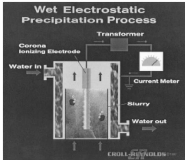
Because wet ESPs operate in a wet environment in order to wash the collection surface, they can handle a wider variety of pollutants and gas conditions than dry ESPs.
